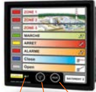
Voltage presence LED «LEDs Test» button Control button
