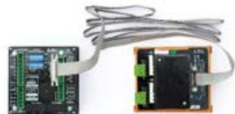
M0901 Card «report relay» DIN type connected to the J1905S panel
